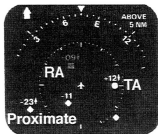
FIGURE 1 Standard TCAS visual symbology. The proximate traffic symbol is shown on an actual display as a white-filled diamond, the TA is shown as an amber-filled circle, and the RA as a red-filled square.
