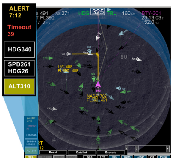
Figure 5. Display of automated conflict resolutions (enlargement shows 3 maneuver options).
