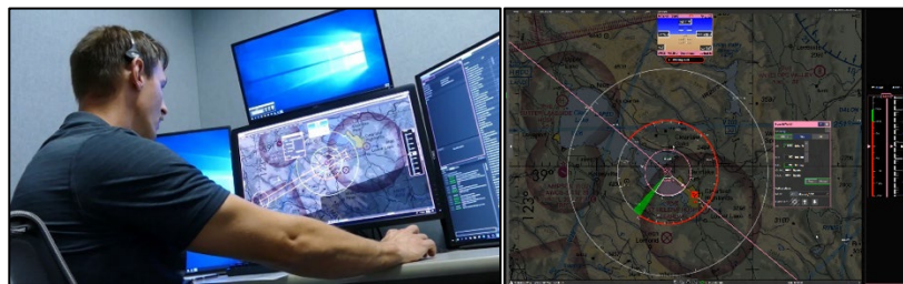
Fig. 11 Uncrewed, ground control station configuration for previous ACAS X_U study. Remote pilot situated in front of Tactical Situation Display with top-down view of aircraft and airspace.
