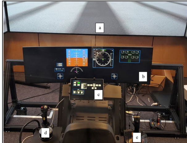
Fig. 1 Pilot displays and controls: (a) Out-of-window views, (b) Electronic Flight Displays, (c) Mode Control Panel, (d) Left inceptor, (e) Right inceptor.
