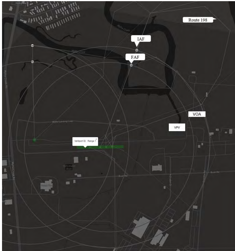
Fig. 19 Vertiport design with VOA/VPV rings, IAF, and FAF.
