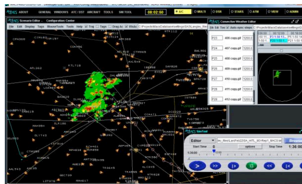
Figure 7. Aircraft, weather and trajectories displayed in the Scenario Editor. The time control on the bottom right is set by the small blue triangle to display aircraft and weather at their positions at any time into the simulation.
