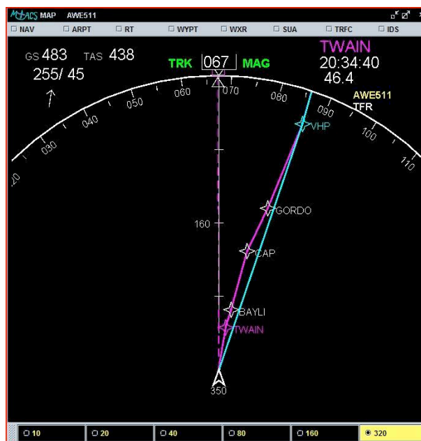
Figure 9. Air-side FMS active and modified trajectories. The magenta trajectory is the active trajectory. The cyan trajectory is a modified trajectory that goes directly to waypoint VHP.
