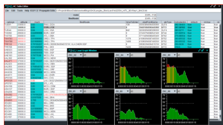
Figure 8. Aircraft and load tables in the Scenario Editor. The load graphs in the center right bottom are the number of aircraft in various sectors in 15 minute time slots as projected by trajectories generated from flight plans. The table in the background contains all the initial conditions for each aircraft, one per row.
