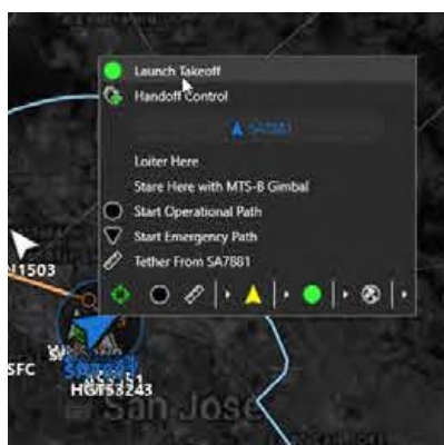
Fig. 3 Context menu used to manually send a takeoff command to a vehicle in the Voice condition.
