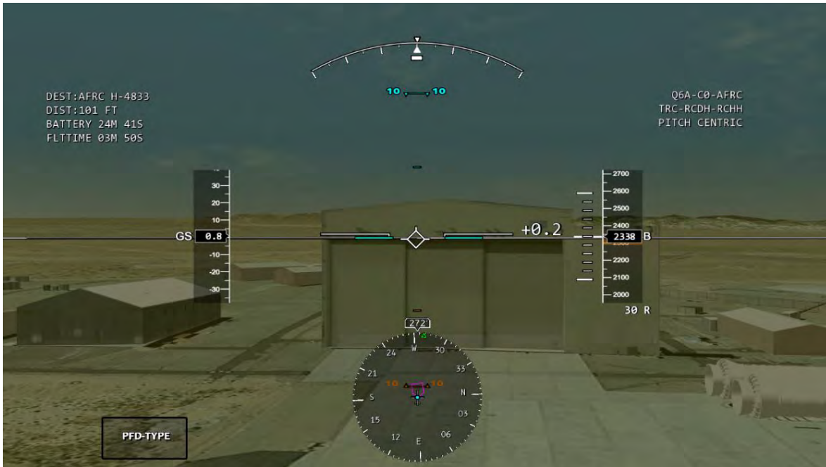
Fig. 17 Approaching Hover Down Condition; 3-D Landing Point No Longer Visible to Flight Crew.
