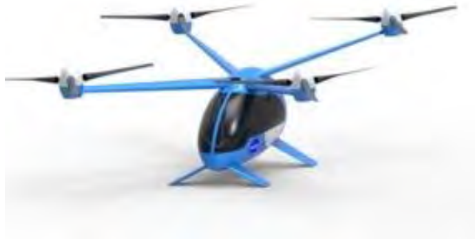
Fig. 3 NASA Six Passenger Quadrotor Concept Vehicle [2].
