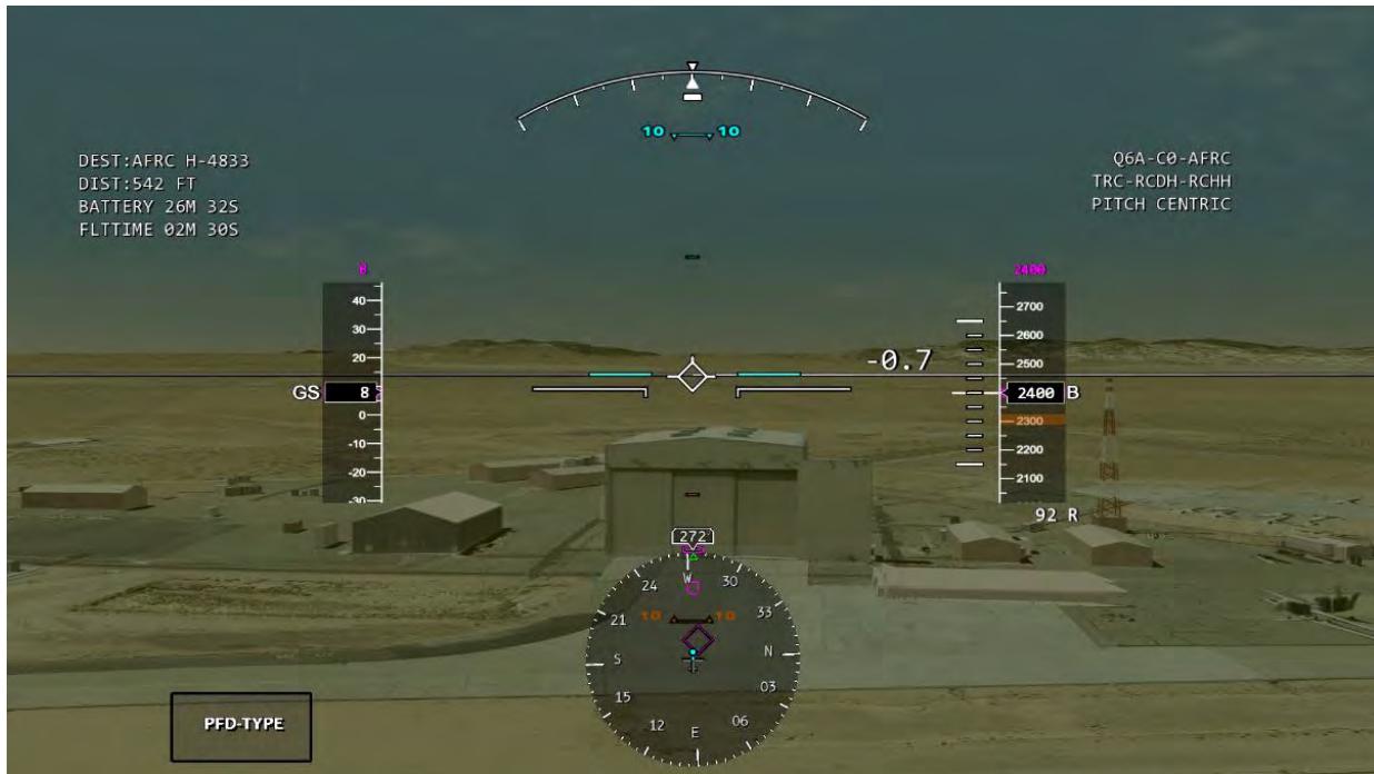
Fig. 16 Approaching Hover Condition; 3-D Landing Point Still Visible to Flight Crew.
