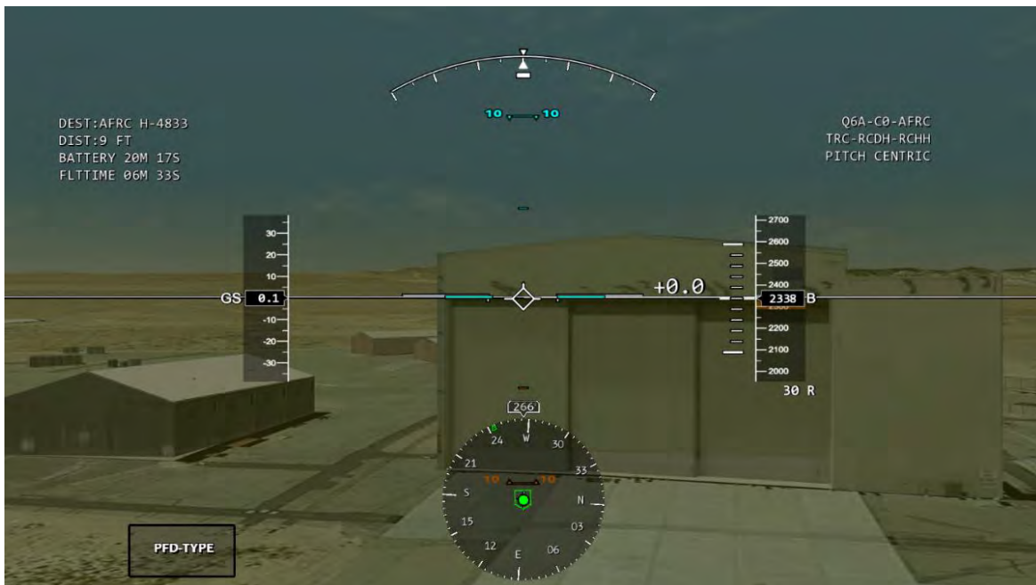
Fig. 18 UAM Vehicle Has Arrived at Landing Point and Now Safe to Hover Down to a Landing.
