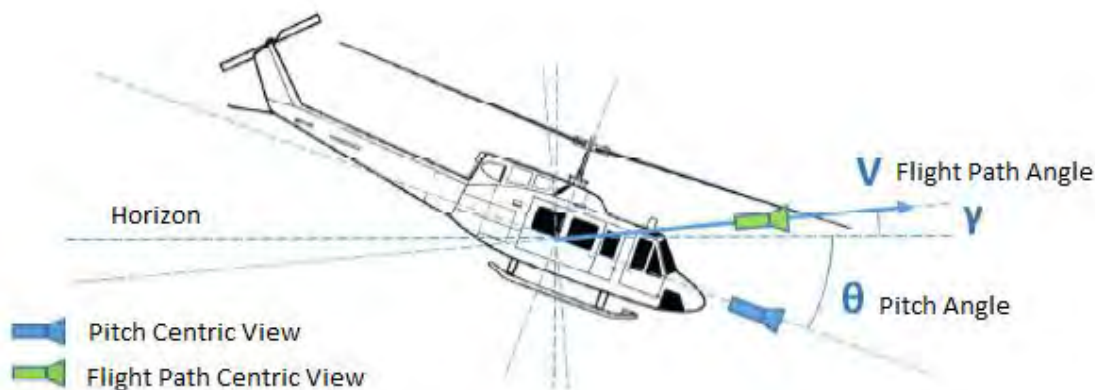
Fig. 21 Pitch Centric vs Flight Path Centric Viewpoints.
