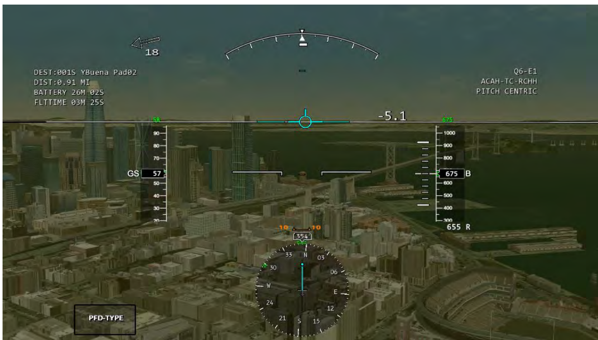
Fig. 13 Enhanced PFD with Integrated Synthetic / Sensor View.
