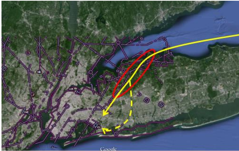
Figure 14: Proposed OPD route for arrivals to JFK 22L and 22R with LGA airspace identified (in red)
