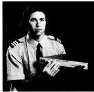
Fig. 1. Ames Spatial Auditory Display (ASAD). The prototype pictured, fabricated for demonstration purposes, works in conjunction with KSC radio communication equipment. It includes an extra switch for a bypass mode that deactivates the spatial filtering, and an extra knob for adjusting left and right ear level test outputs (located on the back of the unit). The EPROMs are accessed by opening the top lid of the unit.
