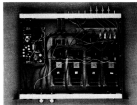
Fig. 2. Internal hardware of ASAD. The four digital boards (bottom right and center) each contain a removable EPROM (mounted on ZIP socket), coder (Crystal CS4215), and DSP chip (Motorola 56001). The analog board (upper right) contains the input filtering and mixing circuitry. Power supply is at left.
