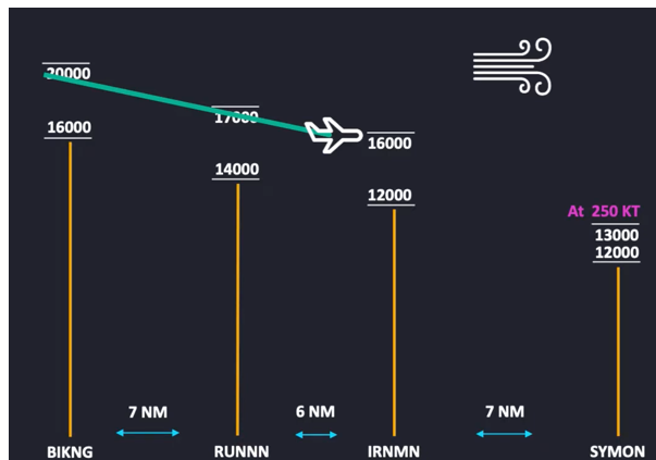
Figure 2. Animation showing vertical profile of airplane flight path with STAR altitudes and distances between way points.
