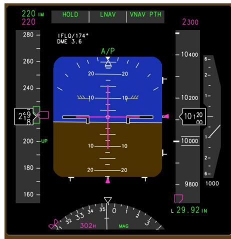
Figure 3. PFD with green FIM target speed (upper left), magenta crew-entered target speed below it, and matching green and pink speed bugs on the speed ‘tape’ (left side).
