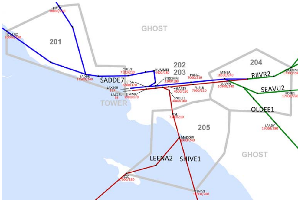
Figure 4. Test Sectors and RNAV Routes to LAX Runways 25L and 24R
