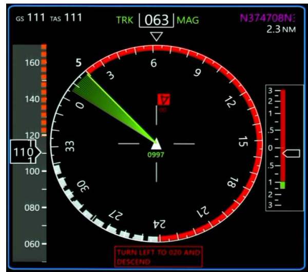
Fig. 2. Screenshot of the ACAS Xr traffic display during a Blended RA.
