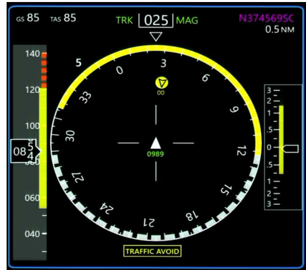
Fig. 3. Screenshot of the ACAS Xr traffic display during a Corrective alert.
