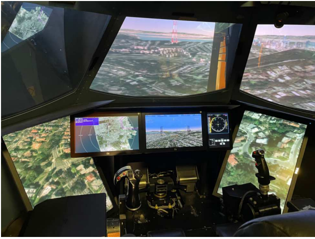
Fig. 1. Picture of the interior of NASA Ames Research Center's Vertical Motion Simulator (VMS) rotorcraft cab.
