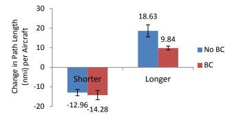
Figure 6. Average change in the path length per aircraft for the aircraft that had longer or shorter final path lengths compared to their original trajectories.
