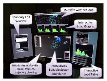
Figure 1. Prototype Airspace Planner station
