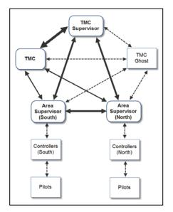
Figure 4. Communication paths between STMC, TMCs, Area Supervisors, controllers, and pilots used in the HITL study (N.B. "TMC Ghost" represented TMUs from adjacent facilities)
