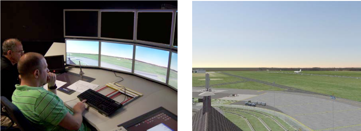
Figure 2. Out-the-window camera or synthetic vision display format.
