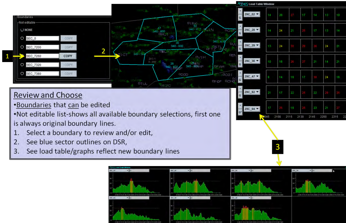
Figure 4. Algorithm-generated configurations available for modification. Traffic load tables and graphs updated with each selection to reflect its impact on the traffic load values for each test sector.
