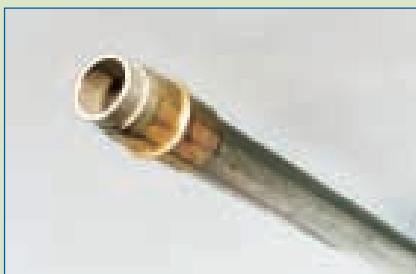
Properly formed (new) tube end: The 'ridge' visible inside the tube end is normal.
