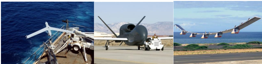
Figure 1. Three examples of remotely piloted aircraft. (a) The 18 kg, catapult-launched Insitu ScanEagle (Photo courtesy Insitu) (b) 6,700 kg High Altitude Long Endurance (HALE) Global Hawk (Photo courtesy Northrop Grumman) (c) AeroVironment Helios Prototype, a solar powered flying wing designed for long-duration, high-altitude missions in the stratosphere (NASA photo, Nick Galante).
