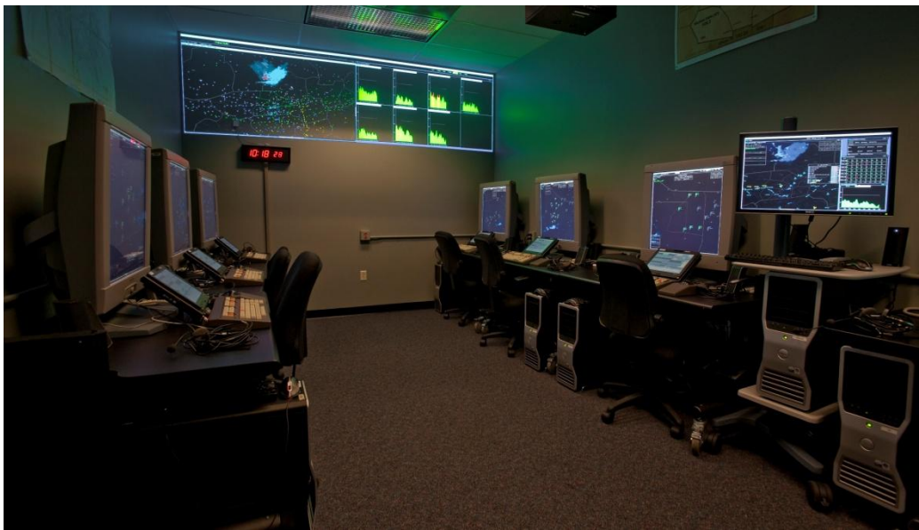
Figure 5. Test area of the AOL showing the six controller and Area Supervisor stations.
