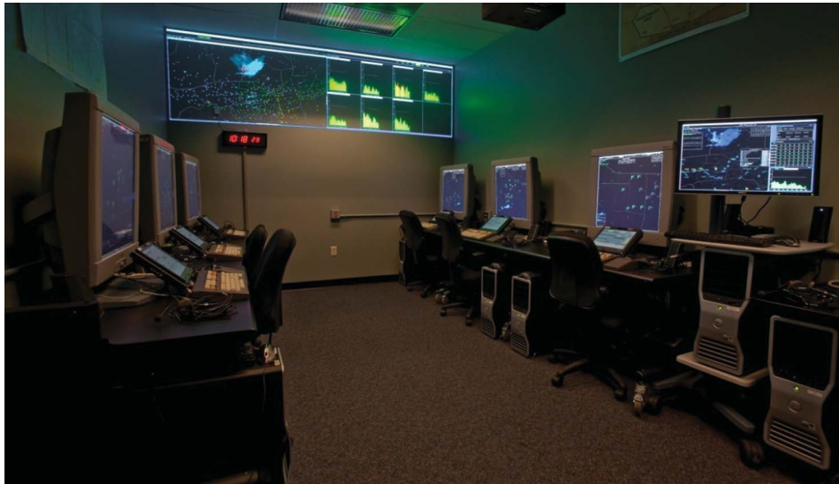
FIG. 3. En route control room configuration with controller and supervisor workstations (color figure available online).
