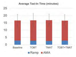
Fig. 6 Average taxi-in time of arrivals going to Terminals A, C, and E. Error bars are standard deviations for total taxi-in times.
