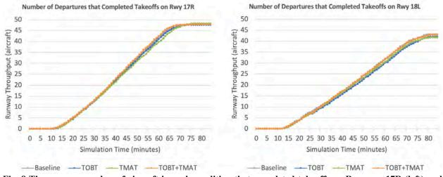
Fig. 8 The average number of aircraft in each condition that completed takeoffs on Runways 17R (left) and 18L (right) over the simulation time.
