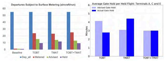
Fig. 4 Average number of departures subject to surface metering per run (left) and average gate hold for departures in Terminals A, C, and E (right).
