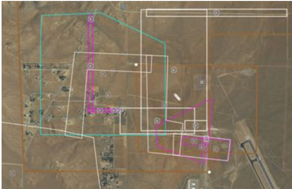
Figure 1b. Example of a test site with multiple GCS area for its vehicles (colored lines denote vehicle volume plan-areas).
