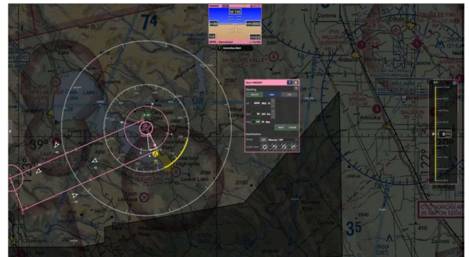
Fig. 1. Screenshot of the VSCS TSD during a Corrective alert. Intruder alert symbol and heading bands are shown near the center-left; altitude bands are depicted on the far right of the TSD.
