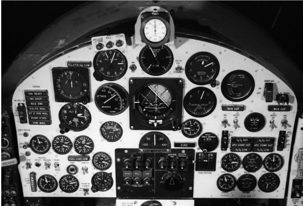
Figure 6.7-1. X-15-3 Original Panel (1960-1965)
