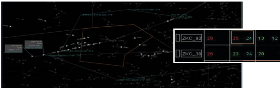
Figure 2.6. Two trajectory changes being performed via lateral trial planning and corresponding Load Table impact values.
