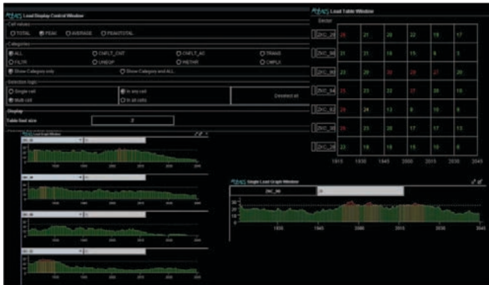
Figure B.5. Load control tool set with load control display window and Load Table and Graphs.
