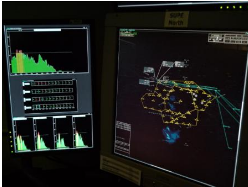
Figure B.18. Planner Display with four route trial plan trajectories pending.
