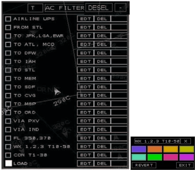
Figure B.12. Example of AC Filter with LOAD selected, showing the available colors for color-coding.
