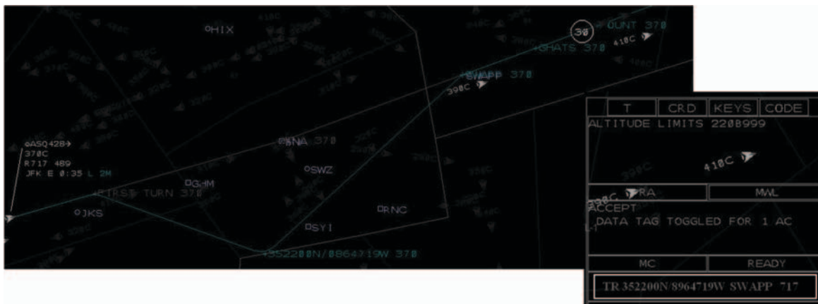
Figure B.24. Example of "TR" command for one aircraft.
