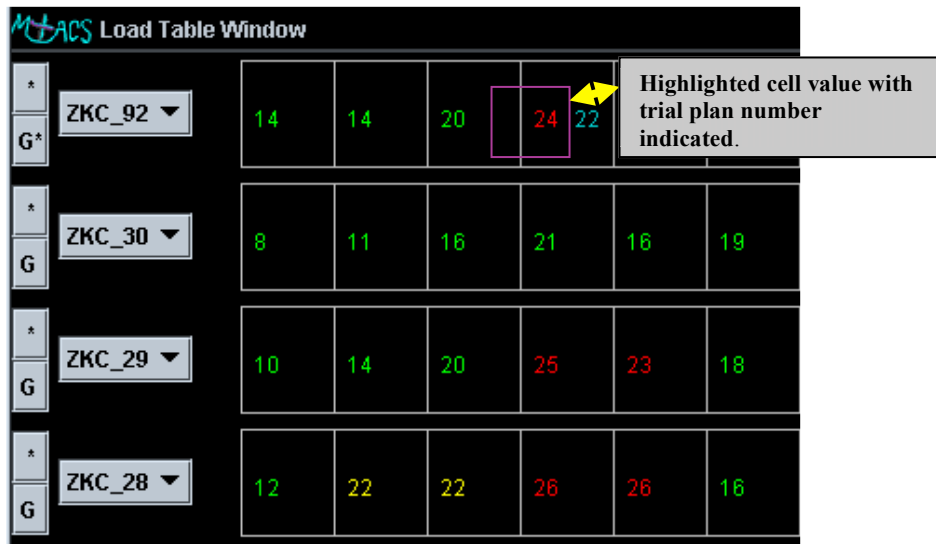
Figure B.7. Load Table Window with sector ZKC_92 selected. There were 24 aircraft that met selected options in the Load Display Control. The cyan number showed the predicted effect of up linking current trial plans, which would reduce the number down by two.
