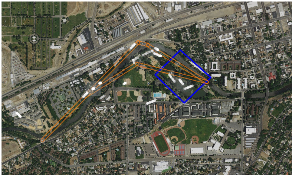
Figure 7b. Example of an event UVR put up during the Reno, Nevada, scenario 2. Event UVR is denoted in royal blue; orange volume is a flight volume showing rogue; white dots are vehicles.
