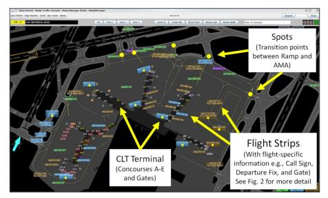
**Fig. 1.** Display of the Ramp Traffic Console (RTC) tool showing the CLT Ramp area with five Concourses (A-E), ramp area (made up of four ramp sectors), and surrounding taxiways and runways. Example "spots," the transition points between the ramp area and the ATC-controlled Airport Movement Area (AMA), are depicted. Each flight is represented by a digital flight strip, which indicates flight-specific information.
