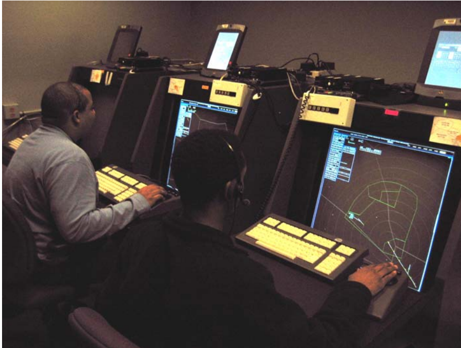
Figure A2. DSR emulation hardware, including high resolution monitors, DSR keyboards & trackballs, and touchpad-controlled VoIP voice communications system.
