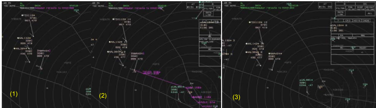
Figure 3.14. MACS/DSR downlink request interface: (1) Ground automation has received a donwlink request from AAL384.Magenta controller cues shown in datablock and status list. (2) Route request accessed by clicking on the magenta arrow is displayed with ground automation feedback (as in trial plan). (3) The controller has approved the request (“ACC” uplink sent to flight crew).
