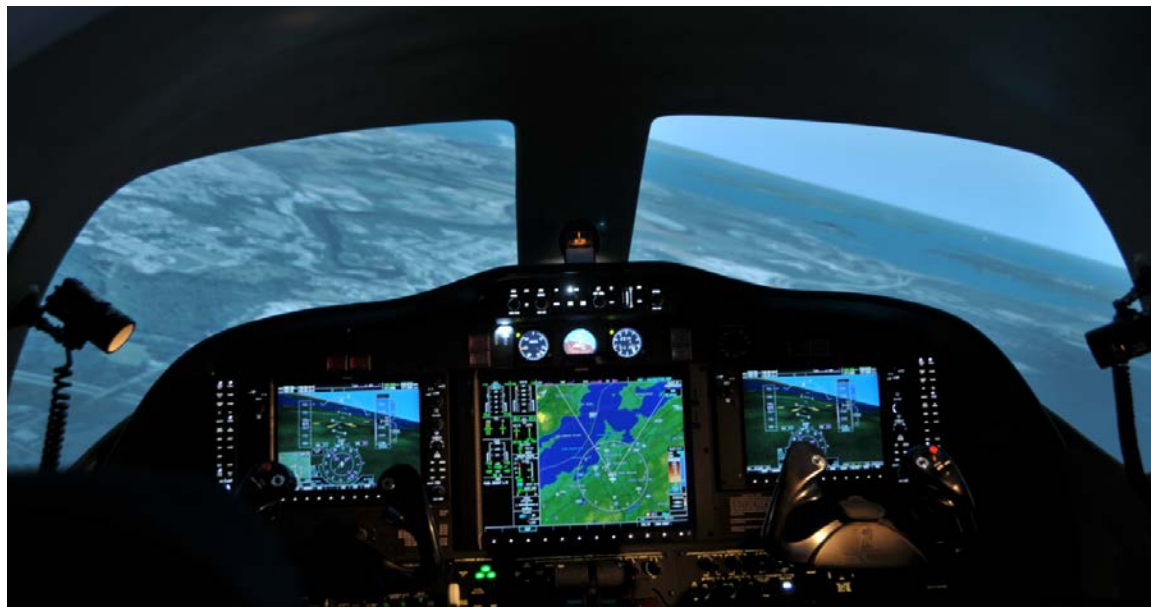
Figure 6. Simulator G1000 avionics suite and out-the-window view.
