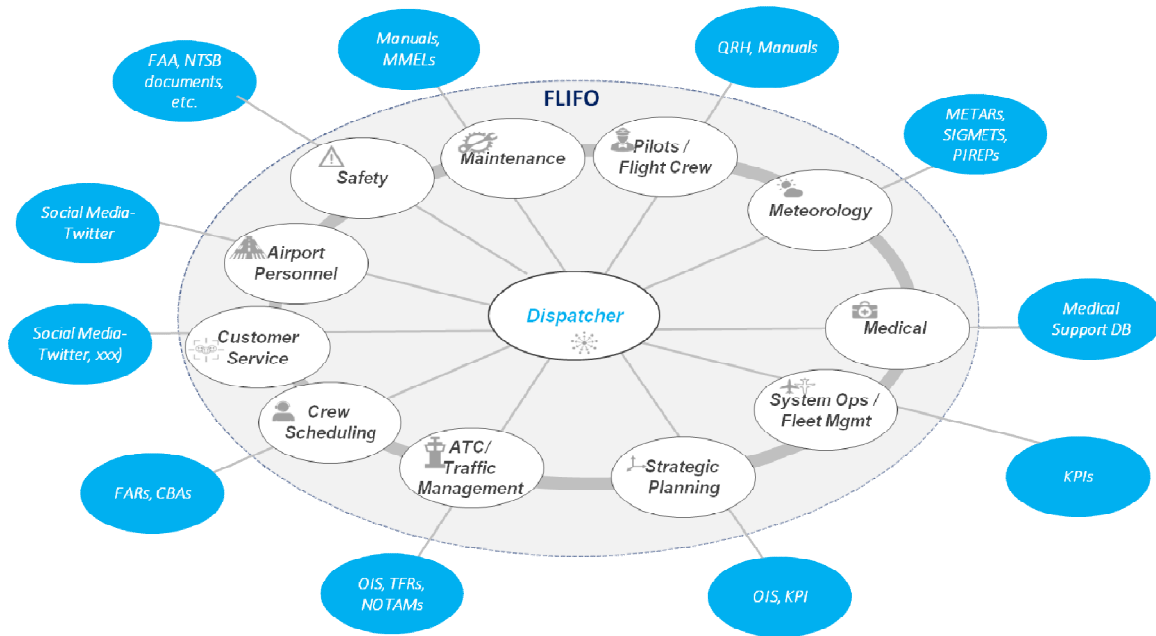
Figure 1: Dispatcher Interaction with Other AOC Personnel and Data Sources (FLIFO = Flight Following)
