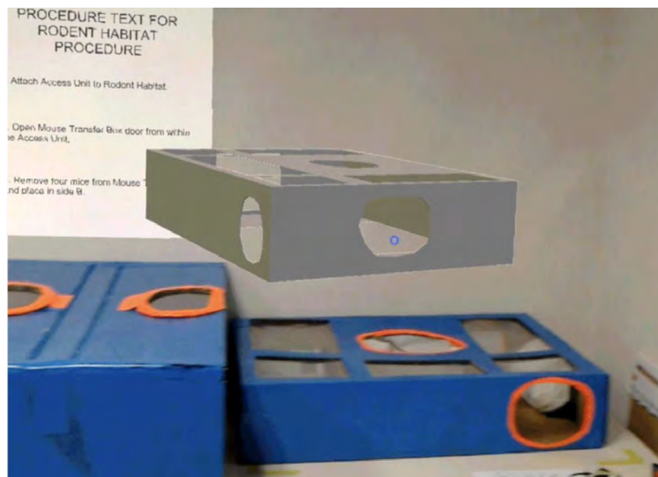
Figure 8. Holographic animations of the rodent research habitat showed users how to complete the task.
