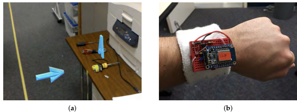
Figure 9. (a) HoloLens holographic overlays. (b) Wristband with ESP8266 chipset.
