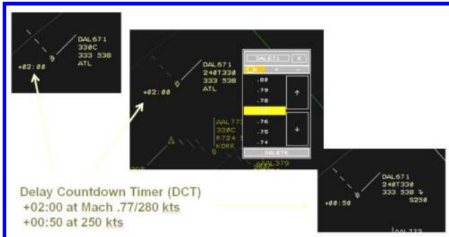
Figure 16: Use of controller entered speed to update the DCT.
