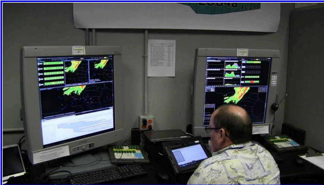
Figure 10: Evaluation of the OASIS advisory tool in AOL with two MACS displays for airspace and complexity assessment and OASIS tablet (center).
