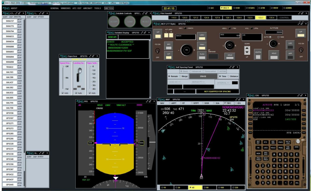
Figure 6. MACS multi aircraft pilot station configured for mid-term environment with integrated data link and airborne spacing functions
