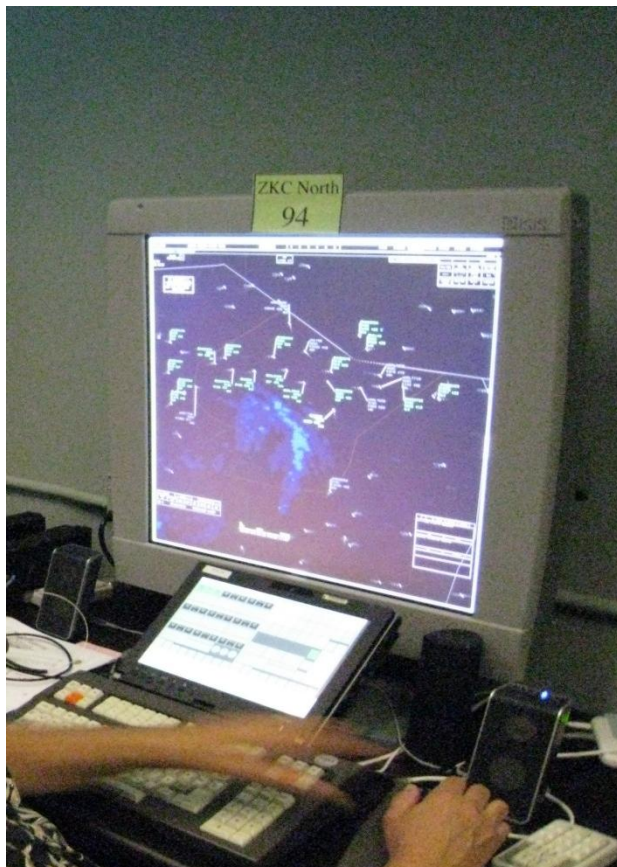
Figure 8. Controller display configured for mid-term (e.g. 2018) NextGen operations at 33% higher traffic density than today'
