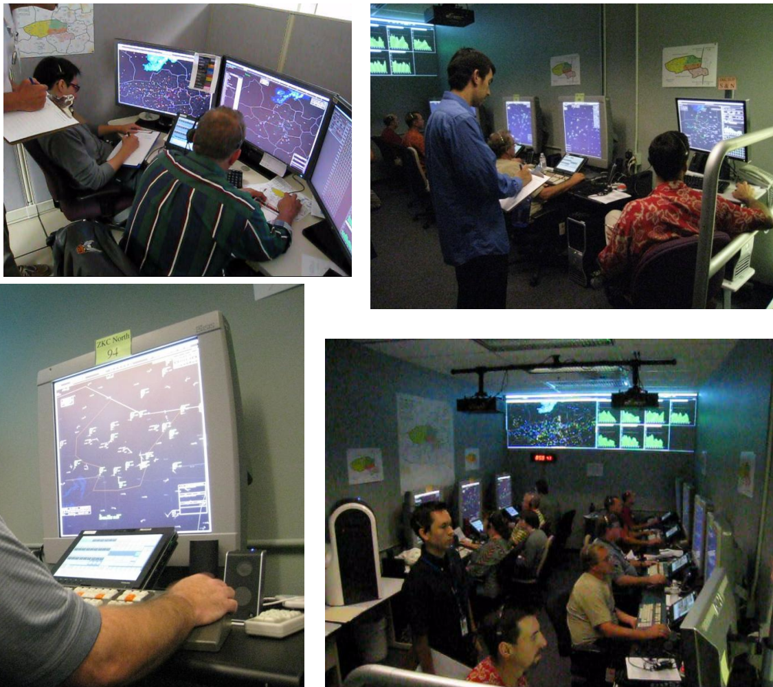
Figure 4. Example participant position in the AOL during Multi Sector Planner simulation in 2009. Clockwise from top left: Traffic Management Coordinator, Area supervisor position (front right), air traffic control area, Center controller workstation with new voice communication system located below the radar display and behind the DSR keyboard.
