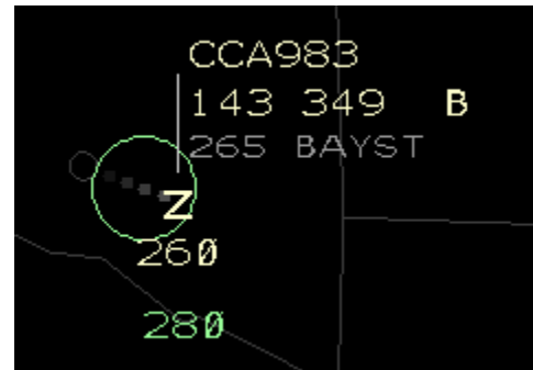
Figure 19. Slot marker circle and speed advisory displayed in the third line of the data block
