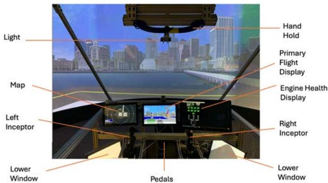
Fig 6. ACEL-RATE Simulator Flight Deck
