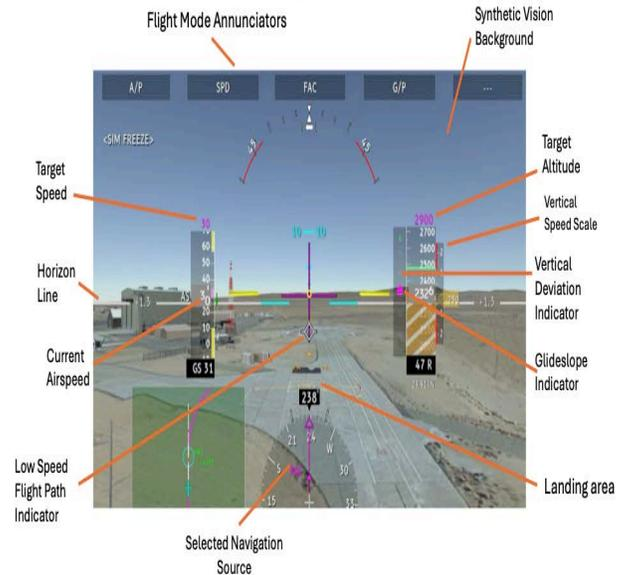
Fig. 7. Primary Flight Display with Synthetic Background
