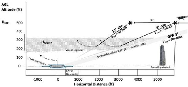
Fig. 16. Profile view of 6- and 12- degree approaches
