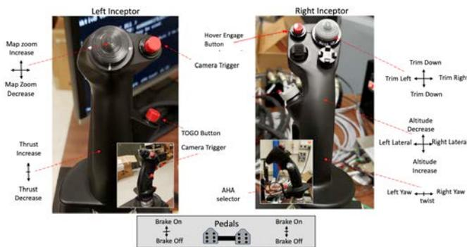
Fig. 19. VMS inceptor controls, grips, and mapping
