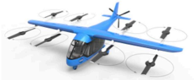
Fig. 2. Lift-Plus-Cruise (LPC) Aircraft
