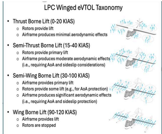
Fig 3. LPC Design Parameters and Lift Sources
