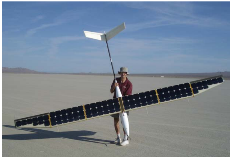
Figure 1. The SoLong UAV developed by AC Propulsion has an electric motor powered by lithium-ion batteries. Solar panels on the wings charge the batteries. In June 2005, the SoLong stayed aloft for 48 hours.
