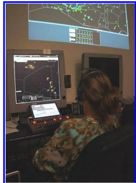
Figure 5: En route controller workstation with ERAM emulation.
